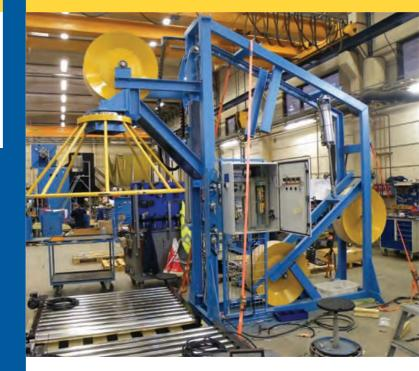
The Vertical Flyer Pay-Off consists of a welded frame on which 3 pulleys with ø500 mm and a gathering cage are mounted on. This pay-off is equipped with a **snarl switch and roller conveyor** for better prepared wire.
