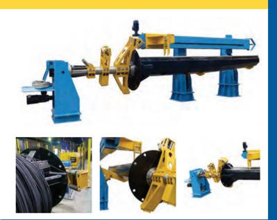
The horizontal Flyer Pay-Off can be equipped with a motor-driven Flyer and Pusher for a streamlined wire preparation process
