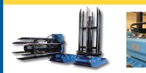
The RPV- TE has a special design for paying-off wire to large drawing or shaving machines for heavy wire.
